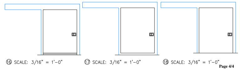
Single Horizontal Electric Slide Door with Backup Casings and Return Jambs
